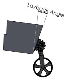
If your transom has a substantial layback angle (10 degrees or more) the second notch can be used to account for this
