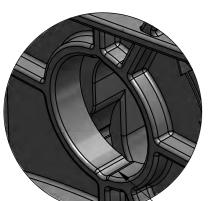
Line upbumps on locking shaft with notches in bracket before insertion
